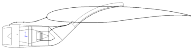
Fig. 1. Proposed way to integrate a CELTIS system using a high by-pass turbofan engine within a supercritical wing
